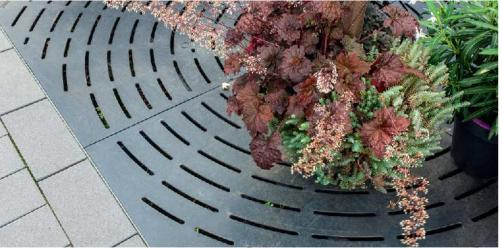
MeierGuss tree grill systems 2.0 enable project-specific solutions to be realised. The cast-iron tree grills are installed with a dip in the middle relative to gutter and street level. This ensures that the soil around the trees is protected without the problem of any differences in height. Local bars and restaurants are able to make full use of almost all the space.
